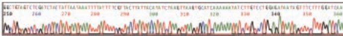
Figure 1. BAC DNA was purified with the PhasePrep™ BAC DNA Kit and sequenced with a custom primer using BigDye® Terminator Chemistry. Sequencing reactions were resolved on an ABI 3700.
