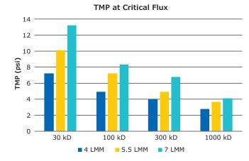
Figure 4. Transmembrane pressure at critical flux.
