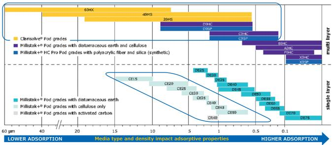
Figure 2. Several depth filters offer robust options for pDNA clarification.
