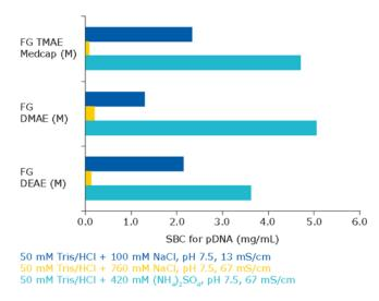
Figure 8. pDNA binding to Fractogel® AEX resins tolerates presence of elevated concentration of  $(NH_4)_2SO_4$ .
