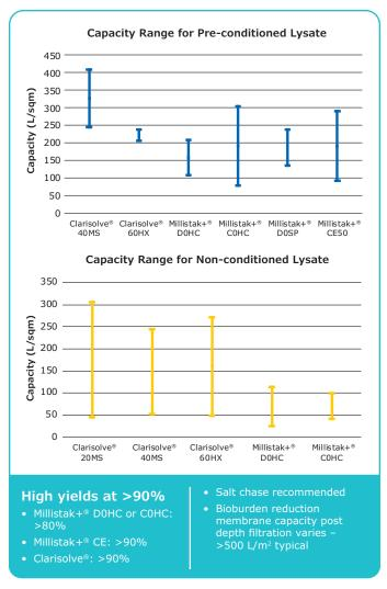
Figure 3. Depth filter capacity ranges for pre- and non-conditioned lysate.
