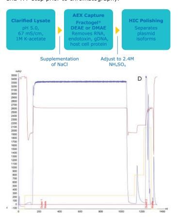
**Figure 7**. Salt supplementation for AEX direct capture eliminates need for pre-treatment and TFF.
