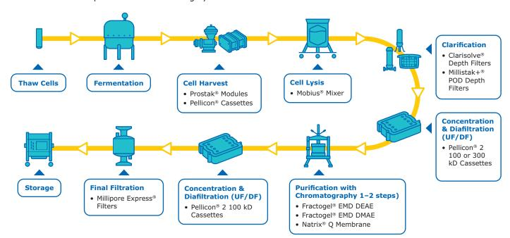
Figure 1. Integrated workflow with capabilities for pDNA purification from harvest to final fill.
