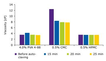
Viscosity of polymeric solutions before autoclaving and after 15, 20 and 25 min sterilization.
