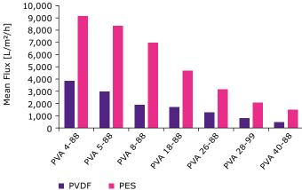
Figure 6.  $V_{\text{max}} \text{ and mean flux of PVDF and PES filters used for sterile filtration of solutions of different PVA grades.} \\$
