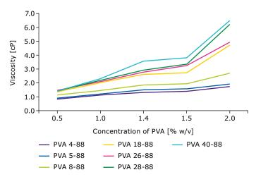
**Figure 3.** Viscosity profiles of different grades of PVA.
