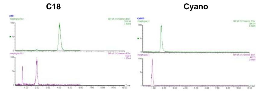
Conditions in Tables 1 and 3. C18 appears to offer the most retention of glucuronide metabolites, without the use of ion pairing.
