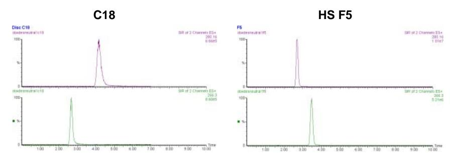
Conditions in Tables 1 and 2. Note the improved peak shape on the HS F5. Also note the elution order change on the HS F5 due to the ability of the nordoxepin to interact more strongly with the HS F5 phase as a result of the loss of a methyl group (secondary amine interacts more strongly than a tertiary amine).
