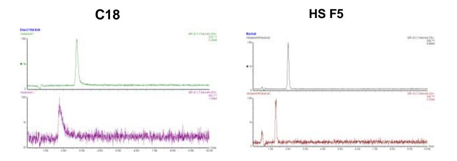
Conditions in Tables 1 and 2. Note the improved peak shape on the HS F5. Note also the sensitivity increase on the HS F5 column due to the improved peak shape.
