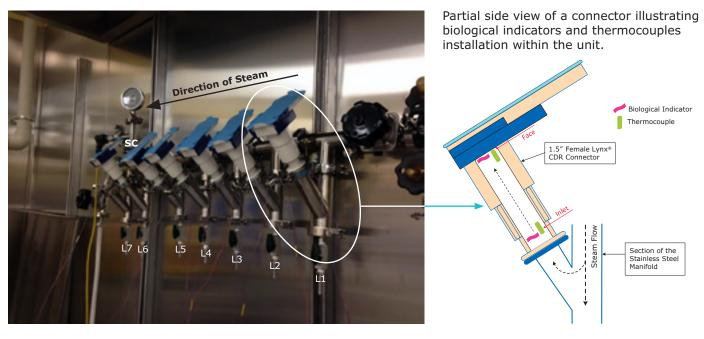
**Figure 1.** System Setup: Stainless Steel Manifold; Installation of Biological Indicators and Thermocouples within a Connector L1-L6: Location ID used for connectors during steaming
