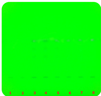
Figure 4. TLC chromatogram for the quantification of glycyrrhizic acid under UV 254nm as documented by the TLC Explorer system.
