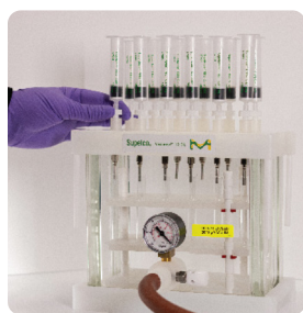
12-Port Visiprep™ DL Vacuum Manifold (57044)
