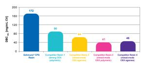
Eshmuno<sup>®</sup> CPS resin provides significantly higher dynamic binding capacities for the model protein Chymotrypsinogen A at elevated conductivity levels compared to benchmark resins.
