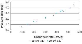
Flow packed in 0.15 M NaCl, 20 cm bed height, 14% compression, running buffer: 0.15 M NaCl
