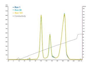
Separation of chymotrypsinogen A, cytochrome C and lysozyme on Eshmuno<sup>®</sup> CPS resin, overlaid chromatograms of run 1 (blue), run 50 (cyan), and run 101 (yellow)
