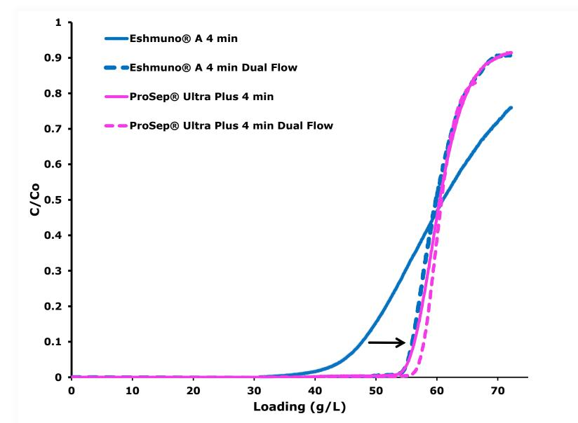
**(Above)** Dual flow rate loading Case 1 increased the steepness of the BT curve and made it comparable to  $ProSep^{(g)}$  Ultra Plus. As a result the DBC at the same effective residence time increased by ~15%.
