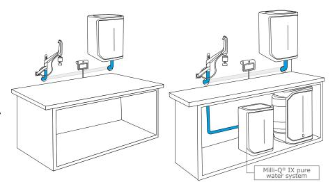
Feed pure water from a pressurized loop or storage tank.
