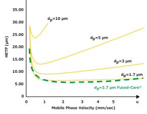
The factors that affect chromatographic efficiency are eddy diffusion, longitudinal diffusion, and resistance to mass transfer, the A, B and C terms respectively from the van Deemter equation.
