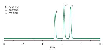
sensitivity and reproducibility using an Ascentis® Express OH5 column and an Evaporative Light Scattering Detector (ELSD) detector.
