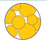
The innovative manufacturing process for Fused-Core® particles produces a very narrow particle size distribution. This allows for the use of larger porosity frits that clogg less, resulting in a more rugged column. Traditional fully porous particles provide a larger particle distribution, requiring smaller pore frits, that clogg more easy.
