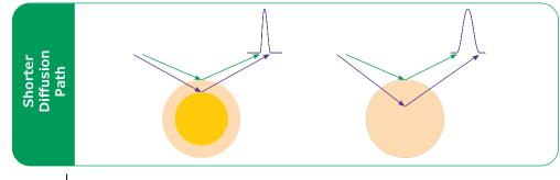
The short diffusion path of the Fused-Core® particle yields sharper peaks than on traditional fully porous particle columns. The minimized resistance to mass transfer, the "C" term in the van Deemter equation, of the Fused-Core® particle provides sharper peaks than traditional porous particles. The short diffusion path also permits the use of higher flow rates without significant peak broadening / loss in efficiency.
