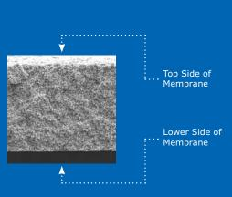
Membranes are 3-dimensional structures full of microscopic pores (Scanning electron microscope image of a cross-section of Immobilon®-P Membrane, Magnification: 500x).
