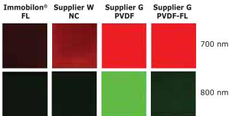
Comparison of background fluorescence observed in PVDF membranes from different manufacturers. Only Immobilon®-FL membrane offers low background fluorescence at both 700 and 800 nm, increasing its ability to used in multiple excitation and emission wavelengths.
