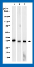
Lysates from NIH3T3 (A) and HepG2 (B) cells were probed with Anti-SOX-9, clone 2B10, ZooMAb® Rabbit Monoclonal (Cat. No. ZRB5535). Proteins were visualized using a Donkey Anti-Rabbit IgG secondary antibody conjugated to HRP and a chemiluminescence detection system. Arrow indicates SOX-9 (~65 kDa).
