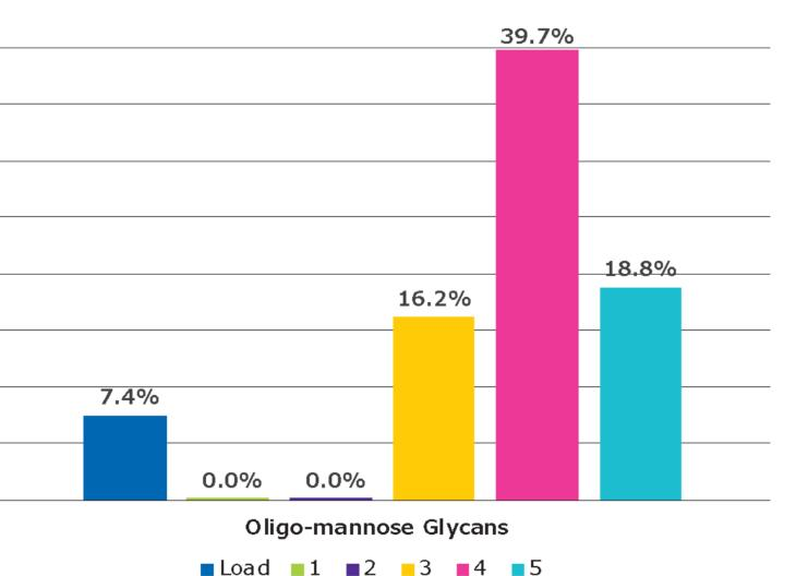
As shown in Figure 3 and 4, using a linear pH gradient elution the separation/enrichment of the oligo-mannose containing glycan species is possible. In the main glycoprotein containing fractions (e.g. fraction 1 and 2), no oligo-mannose variants were detected. Most of the oligo-mannose glycan species eluted in a separate fraction (e.g. fraction 4).
