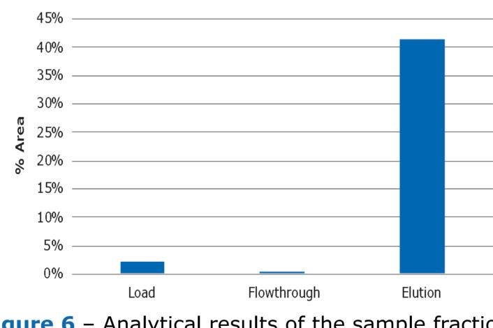
**Figure 6** – Analytical results of the sample fraction characterization using a LC-MS analytical method displayed in quantitative area of analyzed elution fractions (flow through and eluate), including loaded glycoprotein (load) at 10 mg glycoprotein/mL CV loading.
