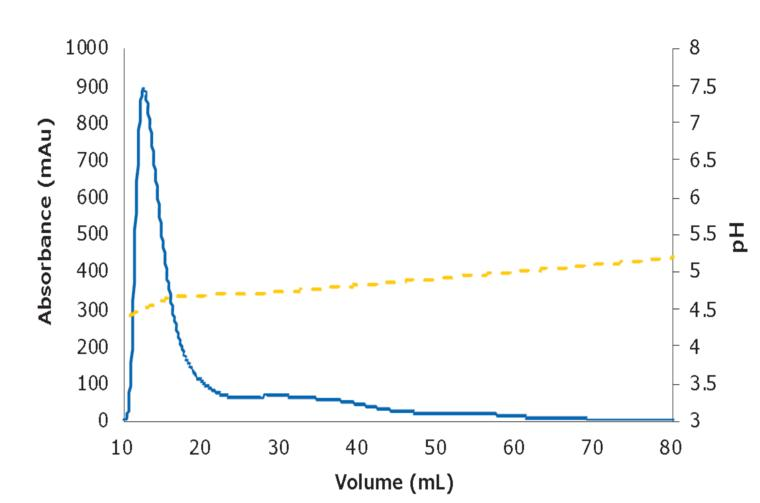
**Figure 5** – Example of pH (yellow) and UV (blue) traces detected for the chromatographic flow-through separation of oligo-mannose containing monoclonal antibody sample loaded to 10 mg/mL CV on the mixed mode cation exchange resin.
