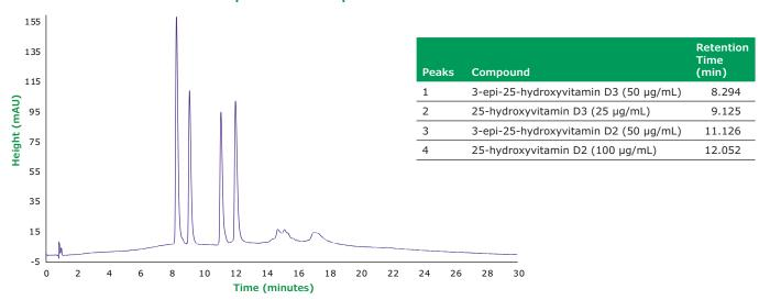
Figure 2: Chromatographic separation of Vitamin D2 and D3 metabolites on Supel™ Carbon LC. Conditions: Column: Supel™ Carbon LC, 10 cm x 2.1 mm I.D., 2.7 μm; Mobile Phase: [A] 2-Propanol; [B] Tetrahydrofuran; Gradient: 0% B to 70% B in 15 min; hold at 70% B for 5 min; Flow Rate: 0.3 mL/min; Column Temp.: 25 °C; Detector: UV, 275 nm; Injection: 2.0 μL; Sample: Vitamin D2 and D3 metabolites mix, varied concentration, ethanol
