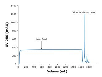
$\label{eq:Figure 8.} \textbf{Figure 8.} \textbf{ Single-step purification with Natrix} \textbf{§ Sb chromatography membrane.}$
