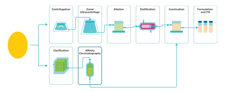
**Figure 10.** Use of affinity membrane chromatography has the potential to significantly reduce the production of egg-based influenza vaccines. Process Reference: Kon, Theone C et al. "Influenza Vaccine Manufacturing: Effect of Inactivation, Splitting and Site of Manufacturing. Comparison of Influenza Vaccine Production Processes." PLoS One vol. 11,3 e0150700. 9 Mar. 2016, doi:10.1371/journal.pone.0150700
