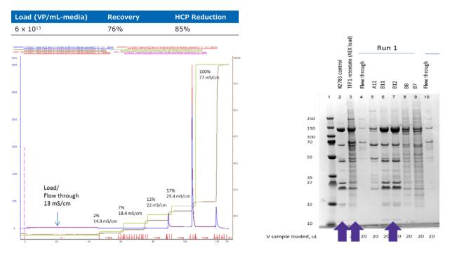
Figure 5. Use of the Natrix® Q chromatography membrane enabled good recovery of the virus and a significant reduction in HCP.
