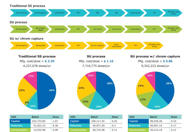
**Figure 2.** Comparison of the cost of goods sold resulting from a stainless steel process, single-use, or single-use with chromatography capture process.
