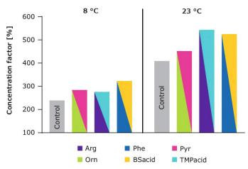
**Figure 7.**Concentration factor of a 10 mg/mL infliximab formulation (100 g) after diafiltration process with or without excipients when reaching an inlet pressure of 40 psi (back pressure valve fully open).
