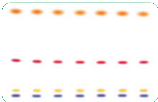
The chromatogram shows four clear separated spots according to Ph. Eur. test conditions and fulfils Ph. Eur. requirements.
