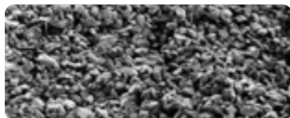
A. Classical silica TLC plate
