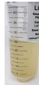
Figure C. LifeSupport™ compacted at the bottom of the centrifuge tube with liquid supernatant removed.
