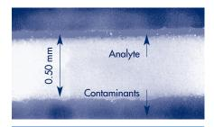
The bed volume of the Empore<sup>™</sup> extraction membrane is thinner yet more efficient than standard sorbent matrices, allowing the use of less elution solvent. The above micrograph shows that analyte is concentrated in a very narrow zone on the membrane surface.
