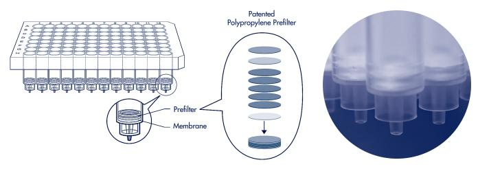
Multi-SPE plates exhibit excellent well-to-well reproducibility. The combination of the patented plate design with the high uniformity of the 3M<sup>™</sup> Empore<sup>™</sup> Extraction Membrane provides consistent recoveries across the plate. The Multi-SPE plate also contains a graded-density polypropylene prefilter secured above the Empore extraction disk. The prefilter is specifically designed to maintain consistent sample flow rates when processing biological fluids.
