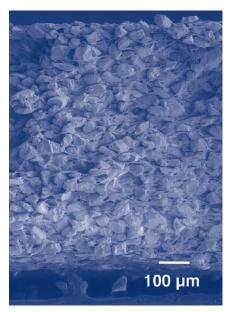
The 3M<sup>™</sup> Empore<sup>™</sup> membrane is composed of chromatographic particles from 40 - 60 µm.
