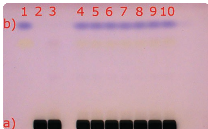
Figure 3. Visualization of the plate under visible light (white light); a) matrix compounds after staining with anisaldehyde sulfuric acid (black areas); b) 2-Methylquinoxaline (blue spot at R_f 80), (reaction product of Methylglyoxal with 1,2-phenylenediamine)
