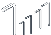
(5) L-Keys Including 12 mm Hex, 1.5 mm Hex, 2.5 mm Hex, 3 mm Hex, T10 Torx
